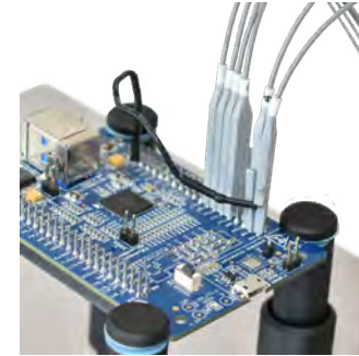
For headers with signals situated together and not enough grounds. A ground lead can be used to connect to a remote ground pin on the device under test.
