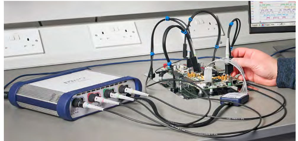
Digital channels connected to a device under test
