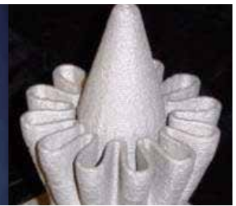
Exhaust Duct Fabricated by LENS System
