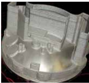
Defense Housing Fabricated by LENS/CNC Process
