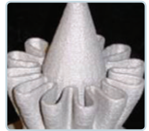
Exhaust Duct Fabricated by LENS System
