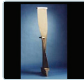
Compressor Blade Repaired by LENS System
