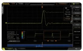
Serial bus trigger and decoding functions (supporting RS232/UART, I2C, SPI, CAN and LIN)
