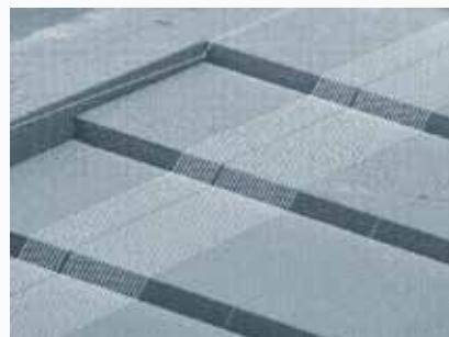
Silver lines printed over a 3D substrate.
