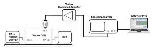
EN 61000-4-6 300 Ohm loop BCI calibration set up using EMCview PRO
