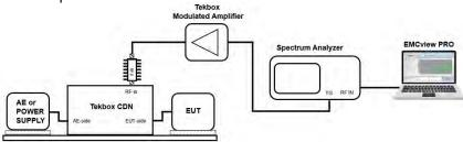
In order to run the immunity test, click the Calibration box in the Immunity Measurement window. Select the calibration file, configure the remaining parameters as desired and click the **start** button.
