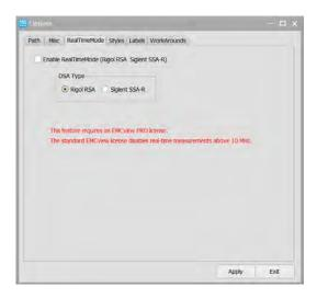
The start button for the measurement will indicate the activation for real-time mode. The configuration section will show two additional segment files, which are used for real-time mode measurements:
