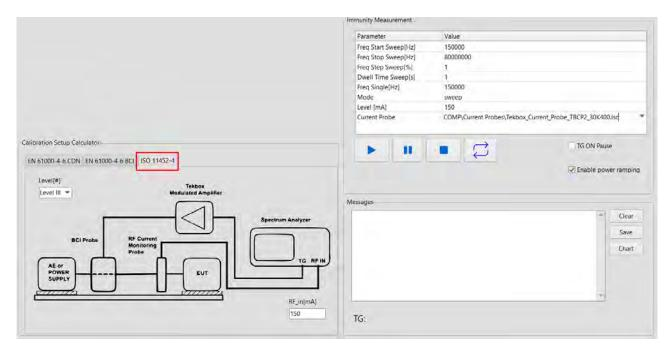
Select the RF current monitoring probe used and the other test parameters and press the Play button. The injected current level will be displayed in a pop-up graph window.
