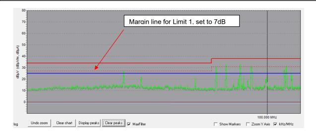
By default, the margins are set to 0, so any peak crossing the limit line would be indicated. Setting margin1 to e.g. 7dB would select all peaks coming within 7 dB close to the limit line of the graph measured with Settings1. Peaks crossing the margin line or limit line can be listed in the in the **Peaks window** by pressing the **Display peaks** button. See chapter 19 on how to manually select peaks and transfer it into the peaks list.
