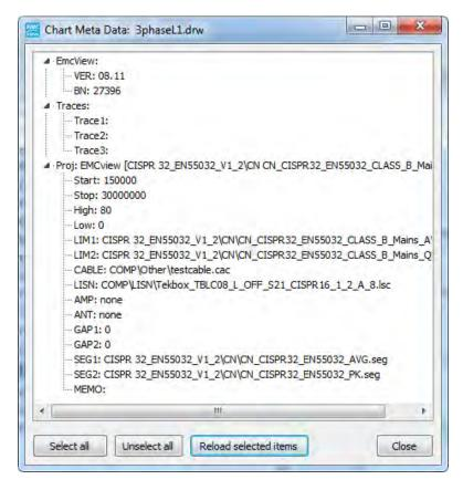
Click **Select all** and **Reload selected items**, if you want to restore the entire set up or make a selection by clicking any of the lines. Note that restoring only works correctly, if all involved files are still present in its original location.
