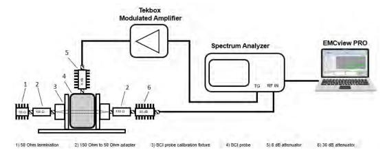
EN 61000-4-6 immunity test set up using a BCI probe using EMCview PRO
