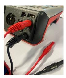
2) Connect the red and black lead to the PRO GTA adapter
