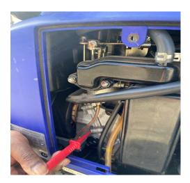
Tester will conduct a Point to Point Continuity measurement between socket earth and stator the result should be less than 1 ohm
