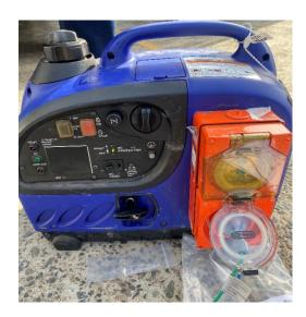
The tester will make a point to point continuity measurement between **socket earth** and **neutral** the result should be less than 1 ohm.
