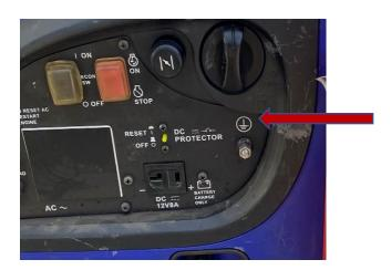
Tester will conduct a Point to Point Continuity measurement between socket earth and Frame the result should be less than 1 ohm
