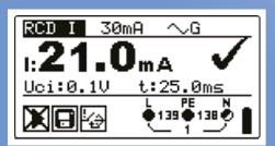
Five RCD testing functions: contact voltage, trip time, trip current, RCD ramp test and AUTO which tests all RCD parameters with one button press. Users can also set test current waveform plus starting
