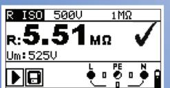
instrument test voltage. Users can set limits for Pass/Fail
