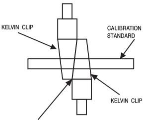
NOTE: Make sure clips are as close together as possible. Use the tips of the Kelvin clips when performing measurements on small diameter wire,
